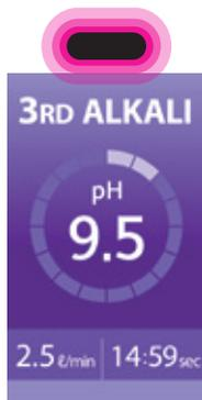
4 When you move your hand close to the proximity sensor the previously selected level (the one with the water droplet on the homescreen) will begin to pour. Move your hand close to the proximity sensor again to stop the flow of water.
