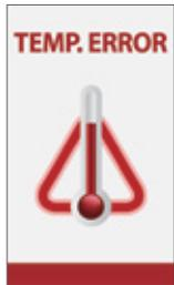
When this is displayed, water inside the unit is hotter than 95°F (35°C). The water supply will then be shut off and the unit will stop operating temporarily. (p. 44)
